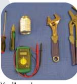
You'll need common plumbing tools and pipe joint compound (or Teflon<sup>®</sup> tape) approved for potable water. You'll also need a circuit tester or voltmeter. Most codes require the water heater to be installed in a metal drain pan. See the Installation Instructions for information about sizing the drain pan and other installation details.
