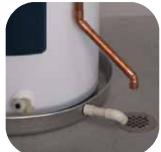
The Temperature and Pressure Relief Valve (T&P) discharge pipe should be terminated near a floor drain with an air gap between the end of the discharge pipe and the drain. Some localities require terminating the T&P discharge pipe outside. In cold climates, we recommend using a floor drain. In all cases, follow the codes for your location. Warning: Do not plug or cap the T&P discharge pipe.
